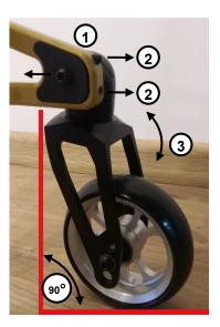
When the position or size of the rear or front wheels is modified, it may be necessary to adjust the angle of the front wheel fork to avoid "fluttering wheels" and ensure a smooth, straight ride.
