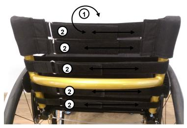
It is possible to adjust the tension of the backrest upholstery so as to be adapt its shape to be user's needs.
