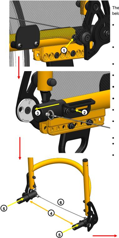
The method of adjusting the seat depth is described below:
