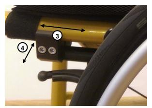
The brakes can be adapted to different types of wheels.
