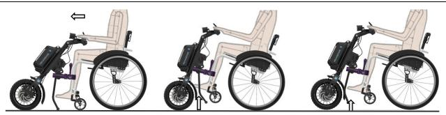
Figure 37. Parking (1), City (3) and Touring (2) positions for Manual Clamp/Lift Devices
