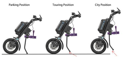
Figure 17. Different positions for the Lift Mechanism
