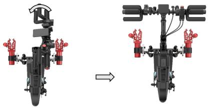
Figure 18. Fixing the Handlebars in the Operating Position.
