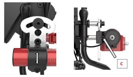
Figure 30. Different positions for Height Adjustment.
