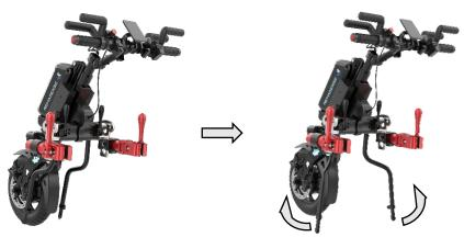
Figure 16. Rotating the Support Legs to the Park Position
