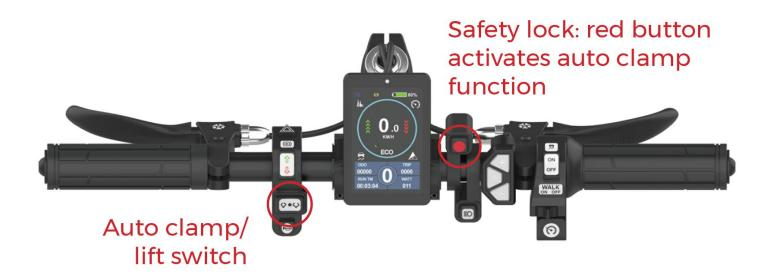
Figure 10. Auto clamp/ lift switch
